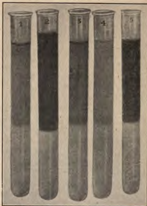
FIG. 48.—Diffusion of colloids into 2 percent agar-agar at the end of a week. 1. Gold hydrosol; 2. silver solution ( Credé ); 3. antimony sulphide solution; 4. arsenic trisulphide solution; 5. iron hydroxide solution.
